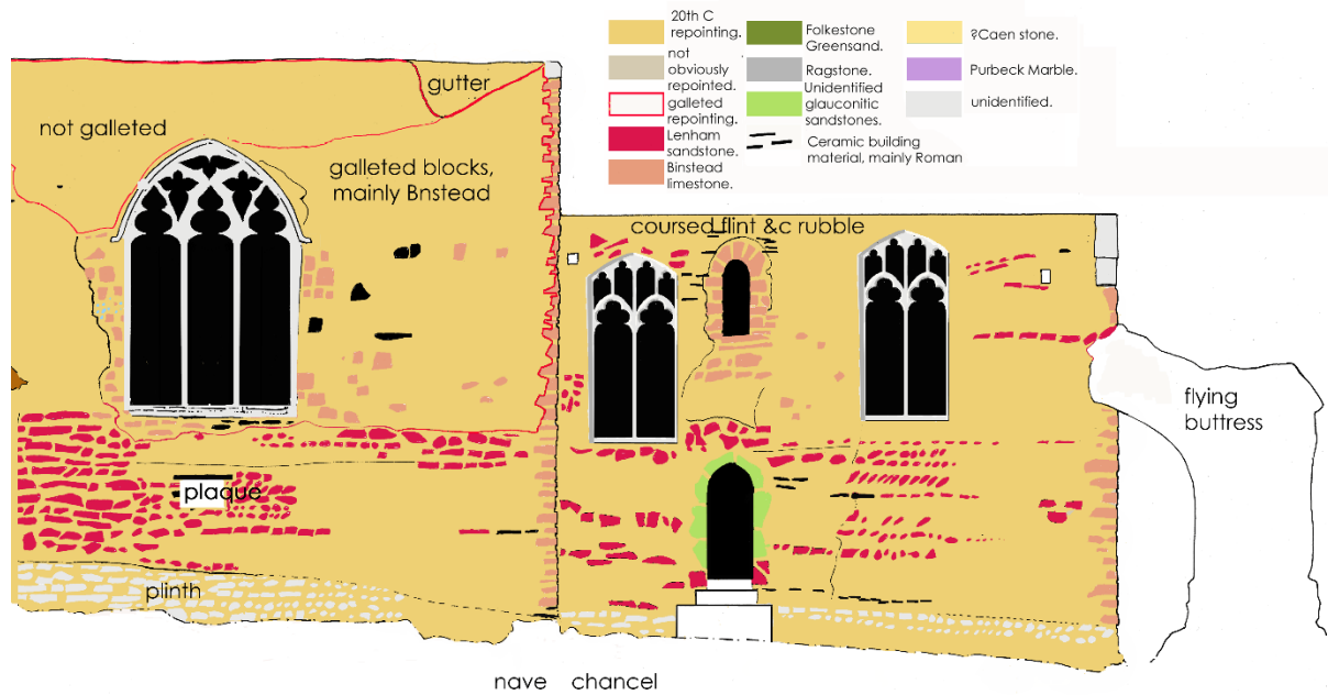
Fig 1. South elevation of church (eastern section) showing geological identifications (scale approx 1:100). Drawing by author based on results of laser scanning survey and select photogrammetry
