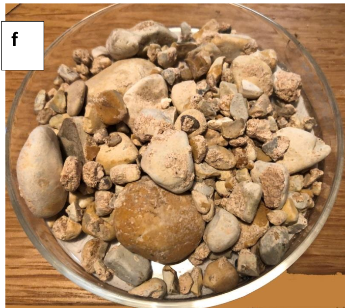
Fig. 6: Lyminge Church mortar Sample 1 (a–c) carbonate replaced plant material; (d–e) marine molluscs; (f) rounded flint beach shingle and gravel. Scales 1mm grid.
