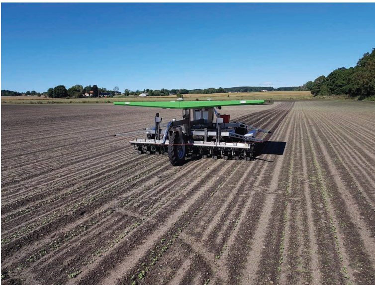
Figure 12 Farmdroid working in newly established winter oilseed rape. The oilseed rape was sown by Farmdroid and is now being inter-row cultivated – another possible application with the machine. Courtesy of Sven Hermansen, SEGES, Denmark.
