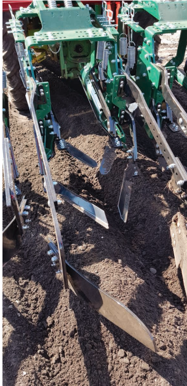
Figure 3 A unit of the OptiWeeder for treating one potato ridge. Courtesy of Bo Melander, Aarhus University, Denmark.
