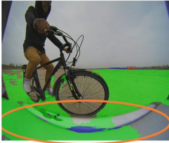
(a) False curb detection (Blue) & Soiling (green)
