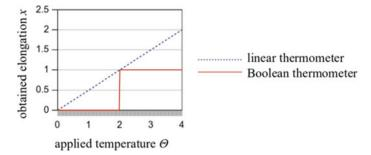
Fig. 1.2 Relationship between  $\Theta$  and x (the transduction function) for thermometers as given in Eq. (1.1) and Eq. (1.2) (scaled values)
