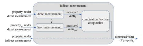
Fig. 7.2 The basic structure of an indirect measurement, including some unavoidable direct measurements (adapted from Fig. 2.11)
