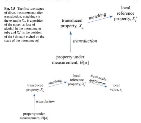
**Fig. 7.6** The first three stages of direct measurement: after transduction and matching, local scale application (in the example  $X_i^*$  is the position of the *i*-th mark etched on the scale of the thermometer and  $x_i$  is a value of position)
