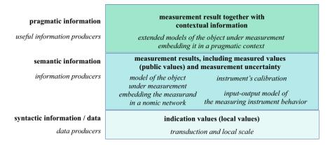
Fig. 8.1 The syntactic-semantic-pragmatic information layered structure in the perspective of measurement
