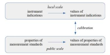
Fig. 7.3 Calibration as a relation of a public scale and a local scale
