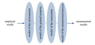
Fig. 4.7 A "lens" representation of the role of models in producing measurement results
