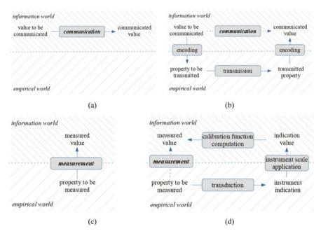
Fig. 4.1 A comparison between communication/transmission (black box (a) and open box (b) models), and measurement (black box (c) and open box (d) models, as elaborated from Fig. 2.10)
