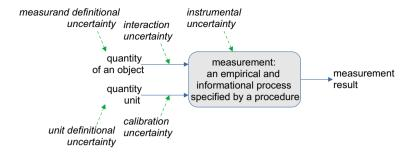
Fig. 3.3 Basic components of measurement uncertainty as related to the abstract structure of measurement (in the case of quantities)
