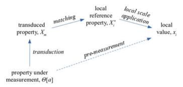
Fig. 7.7 Pre-measurement, as the composition of transduction, matching, and local scale applica-
