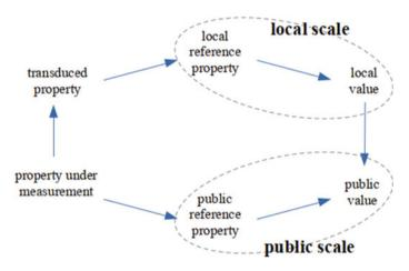
Fig. 7.14 First symmetry in the Hexagon Framework: local scale and public scale
