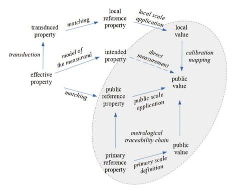
Fig. 7.23 The Hexagon Framework including the definition of the primary scale and its dissemination, and the place (highlighted by the gray ellipse) of calibration uncertainty in it
