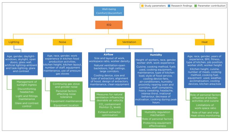
Key: IEQ, indoor environmental quality; BMI, body-mass index; CO<sub>2</sub>, carbon dioxide. **FIGURE 11.1:** Kitchen IEQ framework.
