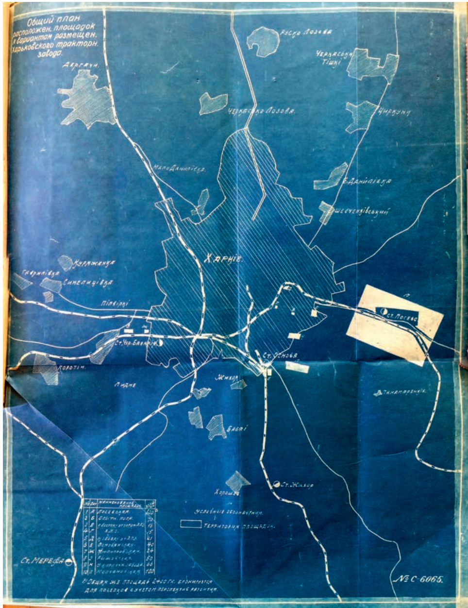
Plate 20. A plan of potential sites for the Kharkiv Tractor Factory, 1929. Report author: Ukrqiprometz. The plan shows the city boundary of Kharkiv (hatched) plus major roads and rail lines radiating from the center. Ten potential factory sites are indicated by white rectangles. Losevo, a preexisting station stop on the southeast heavy rail line out of the city (far right), and largest site by far, was ultimately chosen. TsDAMLMLM Ukrainy, f. 8, po. 1, od. zb. 259, ark. 32.
