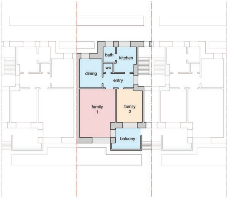
Plate 8. Apartment Type B, a two-room unit, Armenikend test block, Baku, Azerbaijan, 1927. These units were shared by two families, each of whom were given a single private room. Gathering and utility spaces were communal (in blue). Identical Type B units are mirrored on both sides. Architects: Aleksandr Ivanitskii, Anatolii Samoilov, et al. Drawing by the author based on RGALI, f. 2991, o. 1, d. 17, l. 87.
