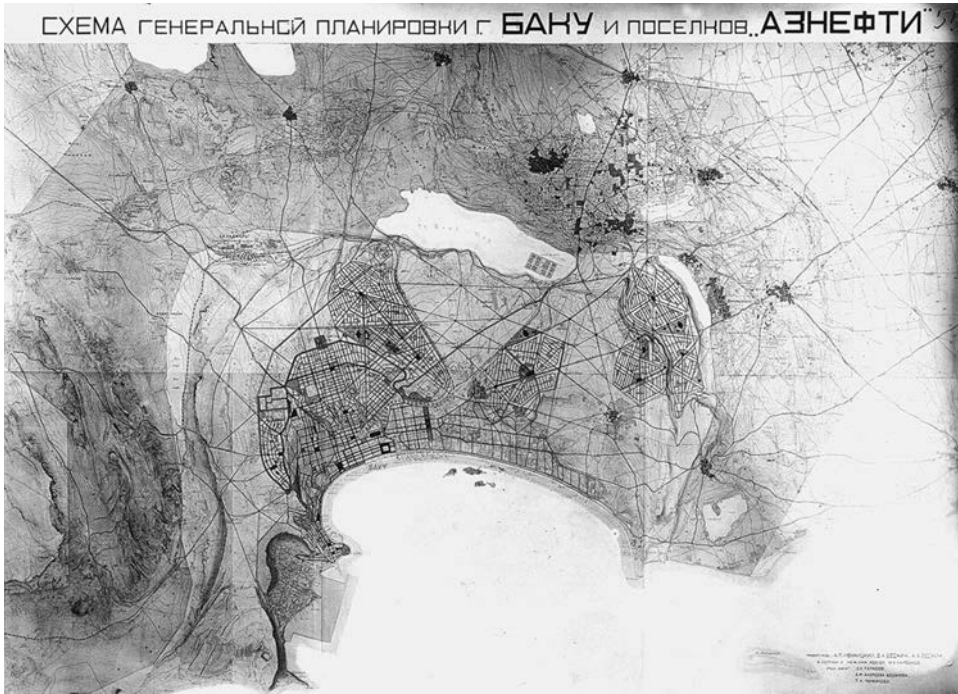
Figure 2.3. A final plan of Baku and Azneft settlements, 1925. Binagady and Montina are a single urban entity, Belogorod lies just northeast of the industrial district of the Black Town, and Stepan Razin sits close to the anticline axis. Planners: Aleksandr Ivanitskii, Viktor Vesnin, Leonid Vesnin, et al. RGALI, f.2 991, o. 1, d. 17, l.55.
