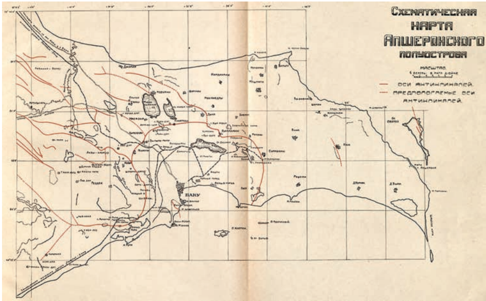
Plate 2. A schematic map of the Apsheron Peninsula. Red lines trace the anticline axes, geological folds along which oil and gas drilling is most productive. Azneft, Obzor Azerbaidzhanskoi neftianoj promyshlennosti za dva goda nacionalizatsii: 1920–1922 (Baku: Azneft, 1922).
