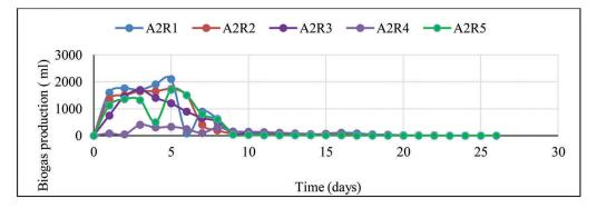
Figure 1. Biogas production rates for the reactors A2 (FS, 2000g; RH and SD particle size, 2mm).
