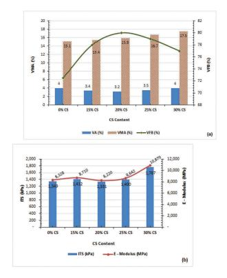
Figure 2. (a) Changes in VA, VMA and VFB in relation to CS content; (b) ITS and E-Modulus results of bituminous mixtures with different CS content at OBC of 4.9%.
