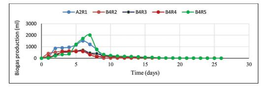
Figure 4. Biogas production rate from reactors B<sub>4</sub> (FS, 3000g; RH and SD particle size, 4mm).
