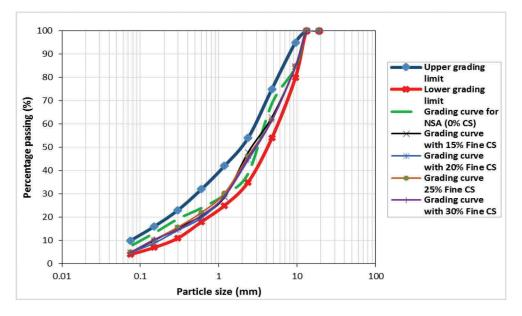
Figure 1. Grading curves for different proportions of CS combined with NSA in relation to the upper and lower grading limits for aggregate with nominal maximum particle size of 14 mm.
