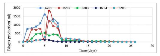
Figure 3. Biogas production rate from reactors B<sub>2</sub> (FS, 3000g; RH and SD particle size, 2mm).
