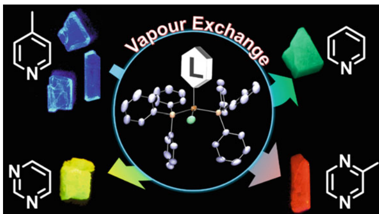
Fig. 4.8 Reversible luminescence color changes of [\text{CuCl}(\text{PPh}_3)_2(\text{L})] based on ligand exchange reactions with N -heteroaromatic vapors. Reprinted with permission from ref. [20]
