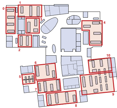
Figure 11.49 Floorplan diagram, with open office areas shown in white, workstations and meeting rooms in blue, and the ten lighting zones servicing workstations in red.
