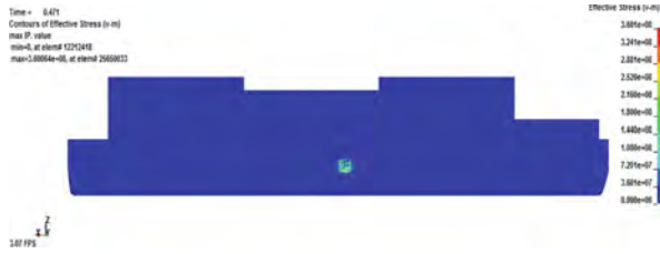
Fig. 11. Equivalent stress cloud diagram of the whole ship at 0.471 s
