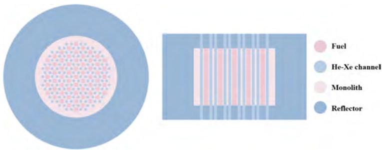
Fig. 2. Schematic diagram of the core
