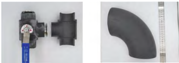
Fig. 3. 3D Printing Nylon-Tungsten Composite Shielding Material
