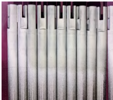
Fig. 11. Weld penetration result
