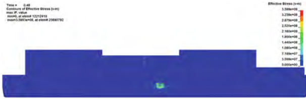
Fig. 14. Equivalent stress cloud diagram of the whole ship at 0.48 s
