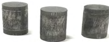
Fig. 4. Coated particle dispersion fuel pellets
