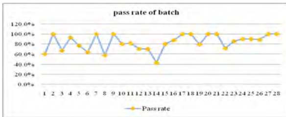
Fig. 1. Fuel rod welding batch pass rate statistics during the experimental phase Statistics
