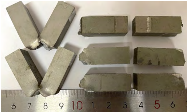
Fig. 3. The impact fracture.
