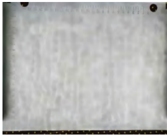
Fig. 2. Macro appearance of sandblasting stainless steel plate.
