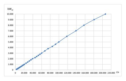
Figure 4.4: Correlation between the CHP-electric power and the biomass input mass flow
