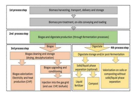
Figure 2.2: Main process steps involved in the operation of a biogas plant (author's own representation according to [27])
