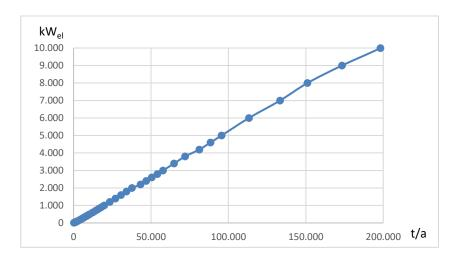
Figure A. 5: Electric power as a function of the biomass input mass flow (E plant)
