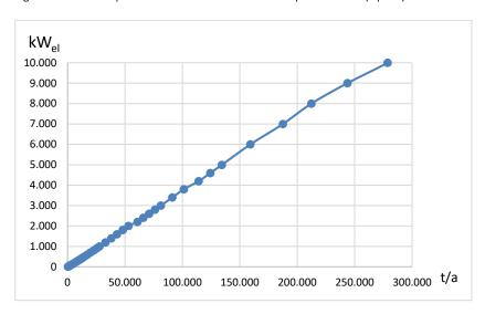
Figure A. 6: Electric power as a function of the biomass input mass flow (B plant)
