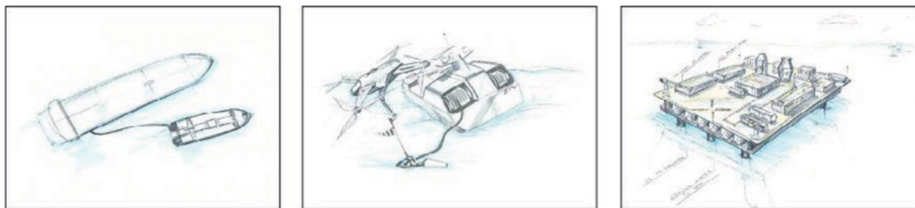
Fig. 20.11 Sketches of zero emission energy distribution at sea. From left to right: Sketch showing ship-to-ship bunkering at sea with zero carbon fuel. Sketch showing drone carrying pilot wire from energy-
