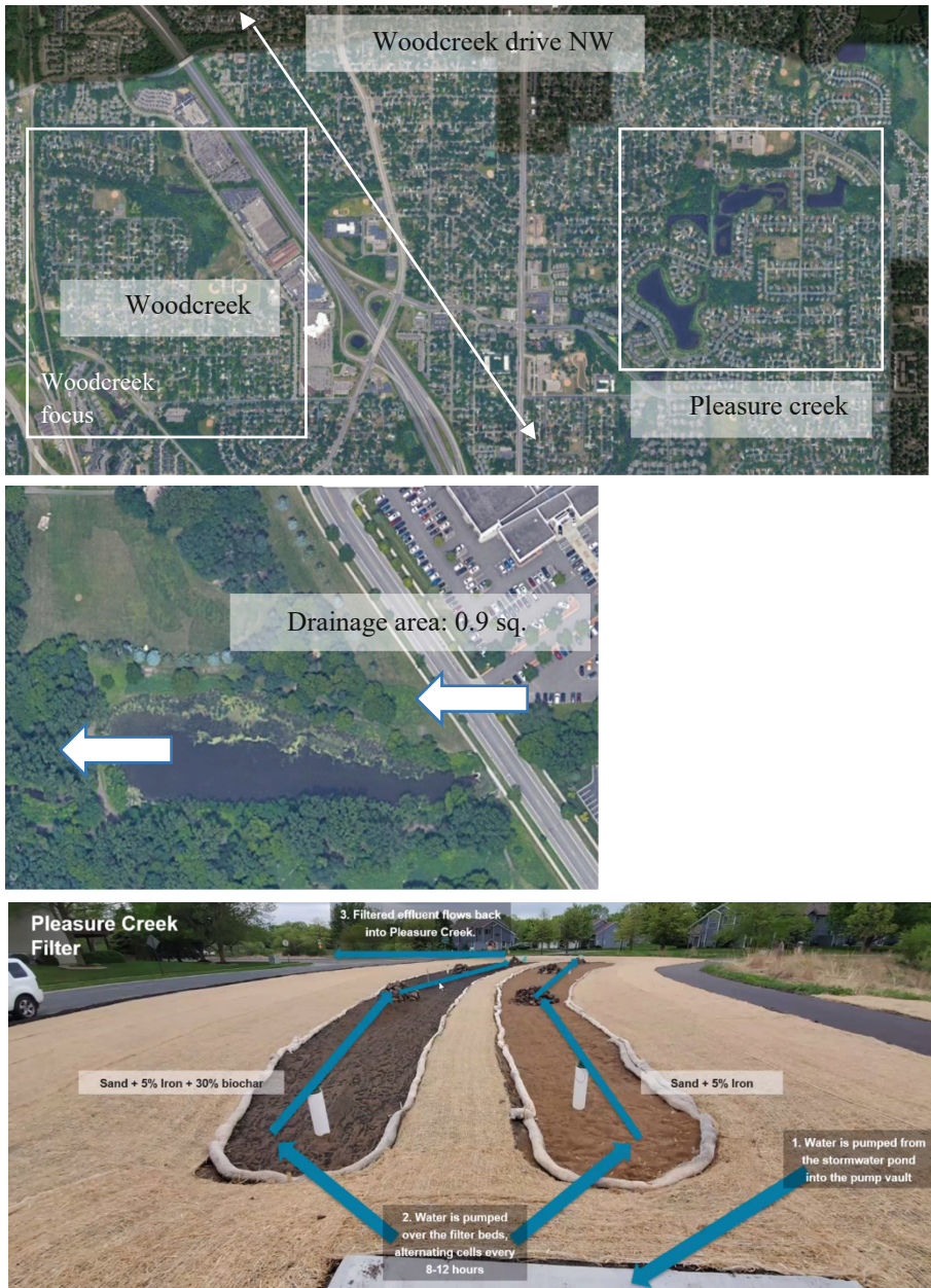
Fig. 6. In the first picture, the Woodcreek drive NW running between the woodcreek and the pleasure creek. In the second picture, a focus on the Woodcreek drainage area used is offered. The third picture shows exactly how the double filter (IESF and BIESF) are applied to the pleasure creek drainage area. The last picture is retrieved from Matthiesen E., and Megow presentation at SER webinar, 22.06.2022.
