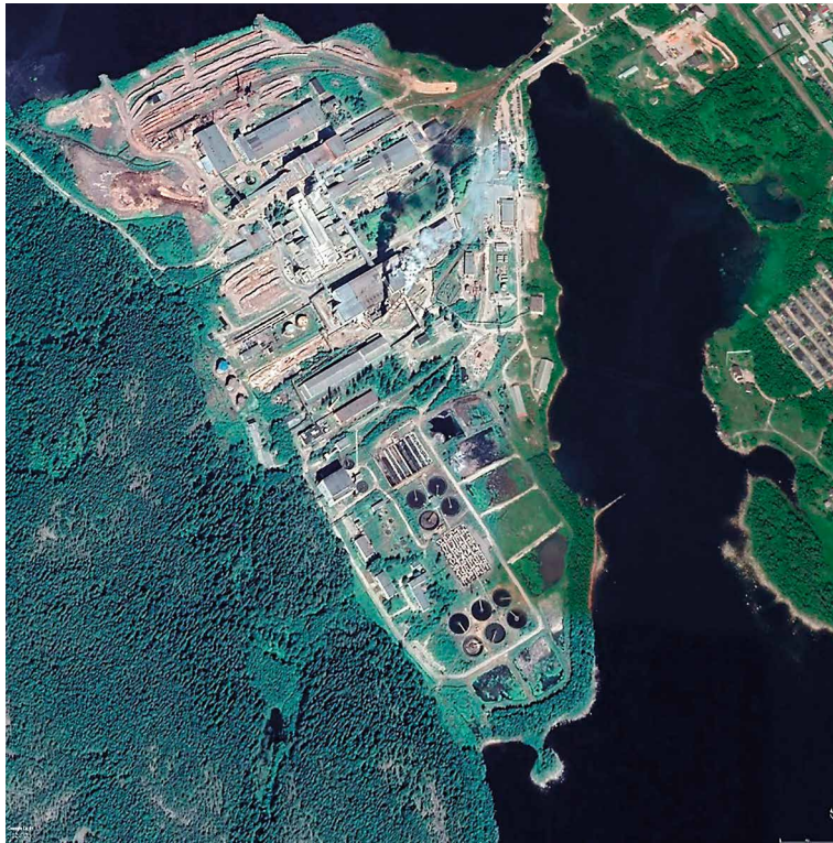
Figure 5. Satellite image of the Pitkyaranta pulp mill, the circular wastewater treatment ponds are clearly visible. Image: Google Earth 2020. © Google Earth 2020.
