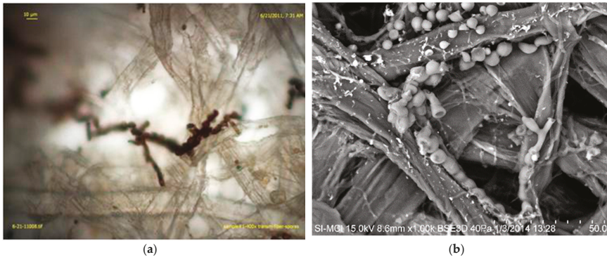
Figure 6.9. (a) Stain type A. In this characteristic pattern of anastomose cells, fungi showed both partial attachment to the surface of paper fibers and partial branching out towards air pockets, which can be attributed to chemotropism. Transmitted light micrograph, scale 10 \text{ }\mu\text{m} . (b) A detailed examination of bio-deposits in the paper matrix showed congregated, single cells of varied sizes. The noticeable indentations in individual spores occurred most likely due to their desiccation. SEM-VP micrograph, scale 50 \text{ }\mu\text{m} . Source: Figure by author.
