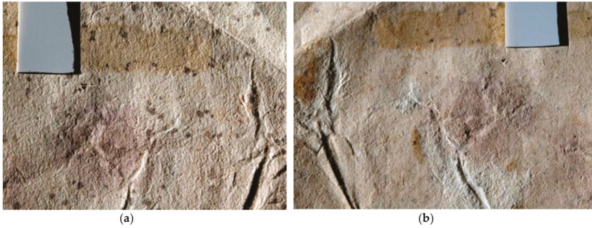
Figure 2.20. (a) Rough surface of paper (referred to as recto, face) with scattered fungal deposits from 17th century Study Sheet. (b) Verso of the same paper, smoother than recto, with a minimal number of fungal deposits. Macro-images 1:1. Source: Figure by author.
