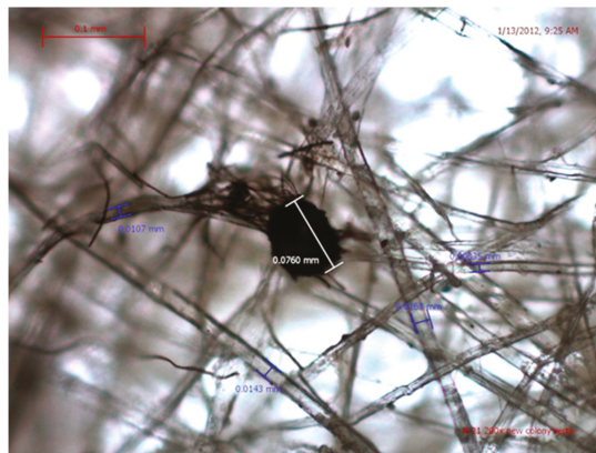
Figure 6.21. Japanese woodblock print, 1847, paper fibers in transmitted light microscope. The fiber diameters ranged from 8 \mu\text{m} to 14 \mu\text{m} ; fibers were well preserved, with smooth surfaces. The black inclusion, 0.076 mm long, is most likely a newly formed perithecium. Transmitted light micrograph, scale 0.1 mm. Source: Figure by author.
