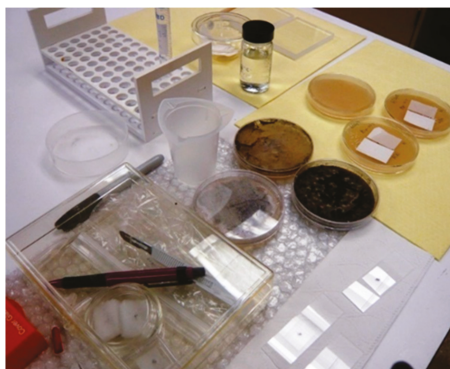
Figure 2.28. The setup of the bio-simulation experiment: Petri dishes, inoculating needle, pure inoculant Aspergillus niger , and sterilized model papers (Whatman 4 and Winsor & Newton). Source: Figure by author.
