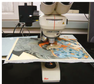
Figure 5.1. The Japanese woodblock print is examined on a support that maintains its flatness. The application of light microscopy poses a challenge for the examination of artworks that cannot be sampled. They require custom-constructed support to carry out an examination. Source: Figure by author.
