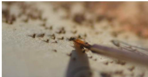
Figure 7.3. An illustration of mechanical removal of Chaetomium perithecia from the surface of paper with a fine brush. This image shows verso of the Japanese woodblock print, Case Study No. 2, on which perithecia were prominently growing. Image taken with Leica D-lux digital camera, scale 1:1. Source: Figure by author.
