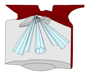
Figure 6.1: Section view of the cylinder of a Bosch internal turbo-charged GDI engine.
