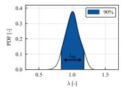
Figure 6.3: Air-fuel ratio  $\lambda$  distribution and evaluation of the homogeneity index  $\lambda_{90}$ .
