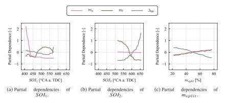
Figure 6.9: Partial dependencies of first start of injection  $SOI_1$ , second start of injection  $SOI_2$  and fuel mass split  $m_{SPIII}$  for the engine characteristics.
