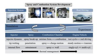
Figure 1.5: Complementary investigations in engine combustion systems [13].
