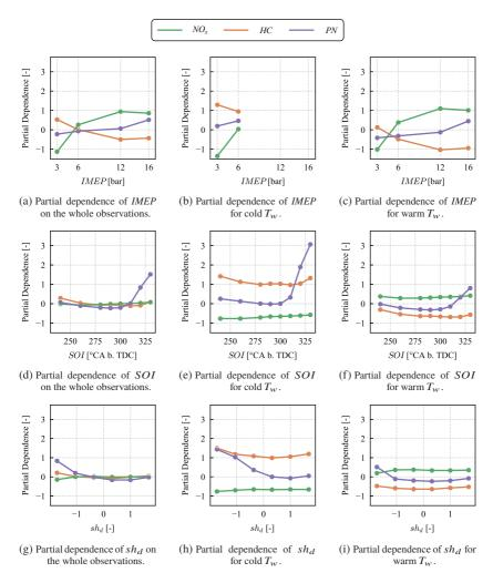
Figure 6.21: Partial dependencies of *IMEP*, start of injection SOI and spray hole diameter  $sh_d$  for the investigated engine characteristics based on the whole observations as well as the warm  $(90^{\circ}C)$  and cold  $(40^{\circ}C)$  cooling water temperature  $T_w$ .
