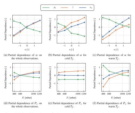
Figure 5.24: Partial dependencies of inclination angle  $\alpha$  and combustion chamber pressure  $P_c$  for the investigated spray characteristics based on the whole observations as well as the warm  $(100^{\circ}C)$  and cold  $(25^{\circ}C)$  fuel temperature  $T_f$ .
