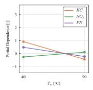
Figure 6.19: Partial dependence of the cooling water temperature  $T_w$  on the emissions.
