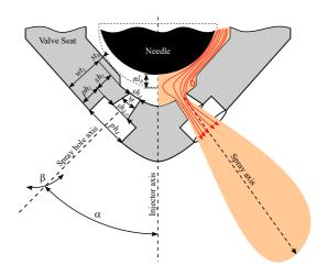
Figure 5.1: Injector nozzle geometry, from [114].
