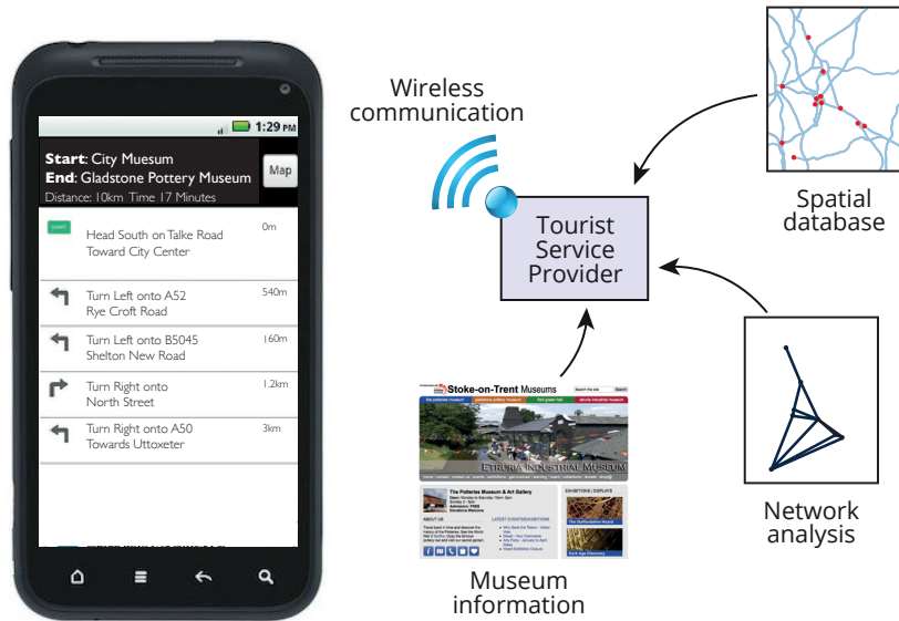
Figure 1.7: Schematic view of a distributed tourist information system
