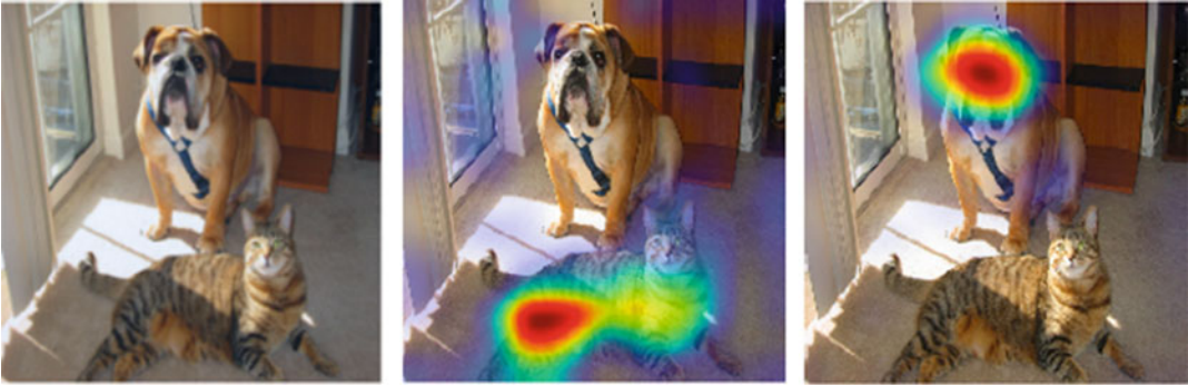
Fig. 8 Grad-CAM explanations highlighting two different objects in an image. (a) the original image, (b) the explanation based on the “dog” node, (c) the explanation based on the “cat” node. ©2017 IEEE. (Reprinted, with permission, from [14])
