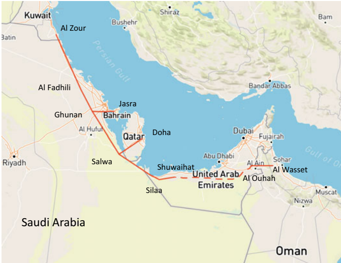
Map 4.1 Approximate route and layout of the GCC interconnection. Source GCCIA https://www.gccia.com.sa/P/the_interconnection_project/55
