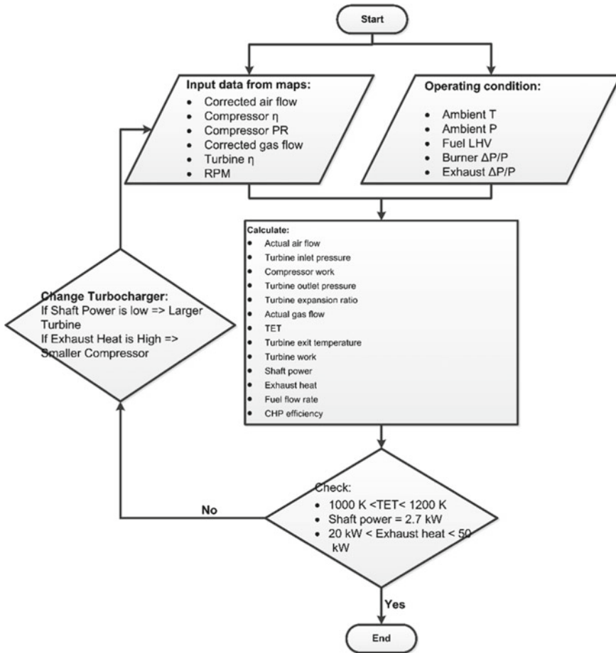
Fig. 33.1 Turbomachinery matching procedure
