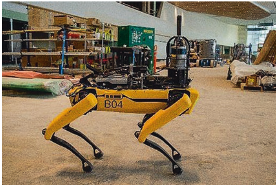
Fig. 8.4 Spot robot for autonomous 360° photo capture. (Image courtesy of HoloBuilder)
