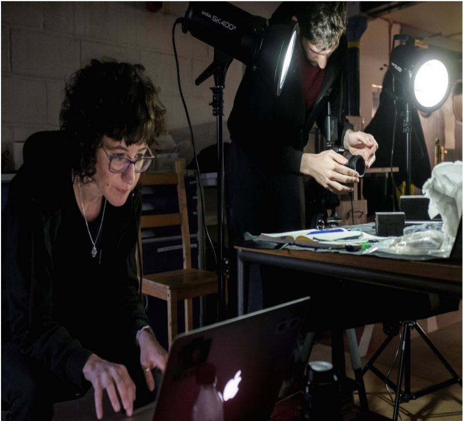
Fig. 3. Physical photographic setup enabling remote triggering and image quality control in real-time to ensure optimum removal of polarised light. Pictured: Clara Molina Sánchez and David Vacas-Madrid.
