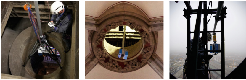
Fig. 19. Shaft tripod with laserscanner lowered through a vault keystone and special support bracket for scans exterior to the spire (right) at Cologne Cathedral 2 .
