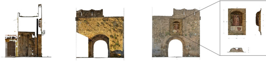
Fig. 2. Point cloud delivered by integration of technologies in “DigiArc” project ( https://www.digiarc.eu ); UAV photogrammetry (top), Terrestrial Laser Scanning and Handheld Scanning (coat of arms).
