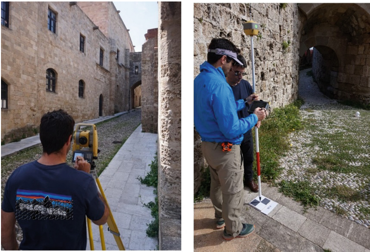
Fig. 4. Measurements with Total Station (left) and GNSS (right) in “DigiArc” project ( https://www.digiarc.eu ).
