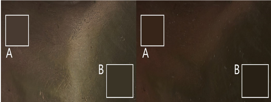
Fig. 12. Comparison between unpolarised (left) and cross-polarised (right) diffuse albedo texture maps for item DC351. Swatches A and B (for both images) are sampled from identical locations and represent averaged colour values for identical areas on both maps.
