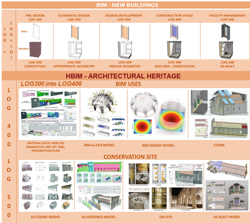
Fig. 12. HBIM turned into preservation aims to support the preservation phases described by the Level of Development (LOD) and the Level of Geometry (LOG): the richness of geometry obtained since from reliable LOD300 (HBIM object model generation – Precise Geometry) supports the LOG400 (HBIM uses) and the Conservation site management (LOG500). Courtesy of ABCIabGicarus (F. Banfi, R. Brumana, C.Stanga)
