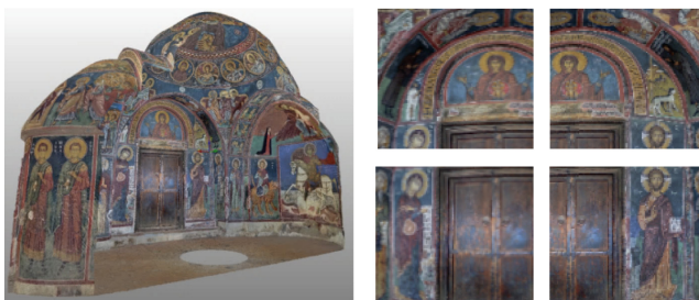
Fig. 6. Color mapped scan (extract) and example of single imagery tiles from the integrated camera sensor with overlaps (right). Example: Panagia Church of Asinou (Cyprus) 1 .
