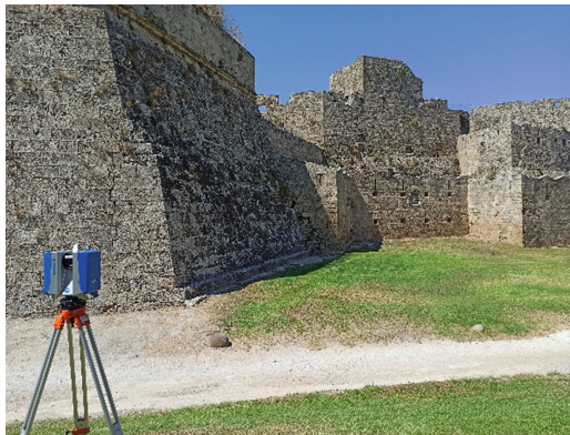
Fig. 3. Terrestrial Z + F 1 laser scanning in “DigiArc” project ( https://www.digiarc.eu ).
