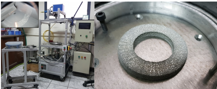
Fig. 2. (a) SGM printing system. (b) SGM printed 316L ring.
