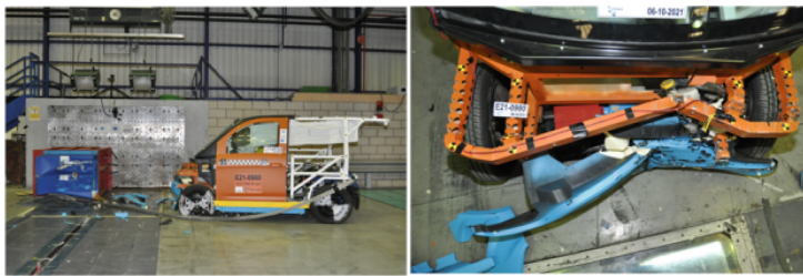
Fig. 4. Vehicle structure after the test according to R94 (left), and detail of the front-end (right).
