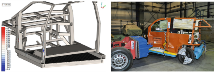
Fig. 5. Vehicle structure after the test according to R95, simulation (left) and real test (right).
