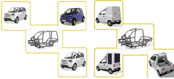
Fig. 1. Modular approach: minimum structural changes lead to different vehicle concepts.
