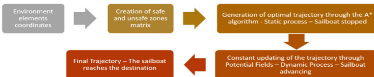
Fig. 6. Trajectory Planning General Algorithm
