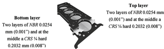
Fig. 2. MLS Gasket Composite Material
