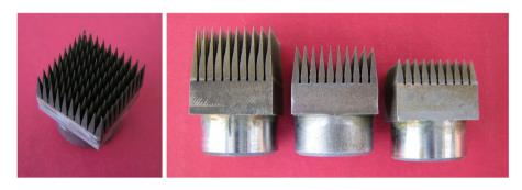
**FIGURE 3.18** Trial geometric structures of the MSC-Scaffold of the prototype resurfacing endoprosthesis of the hip joint manufactured with the use of the wire-cut EDM method with three different heights of the spikes.
