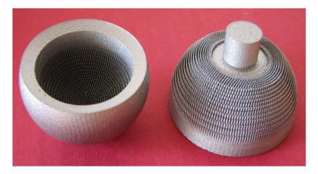
**FIGURE 3.30** Prototypes produced in SLM technology required further precise processing (turning, grinding, polishing, lapping of the cooperating articulate surface of hip joint endoprostheses); visible technological handles allow precise surface finishing.
