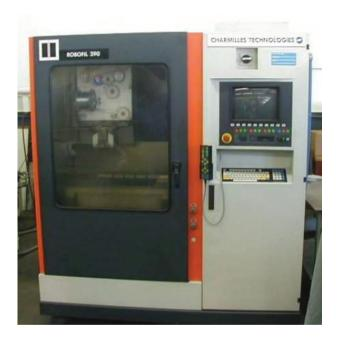
FIGURE 3.16 Robofil 290 EDM machine by the Swiss company Charmilles.
