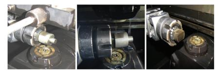
**FIGURE 3.17** Wire-cut EDM of a trial geometric structure of the MSC-Scaffold; the illustrations present the cutting trajectory.
