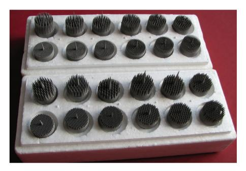
**FIGURE 3.26** A set of 24 preprototypes of the MSC-Scaffold produced by SLM technology.
