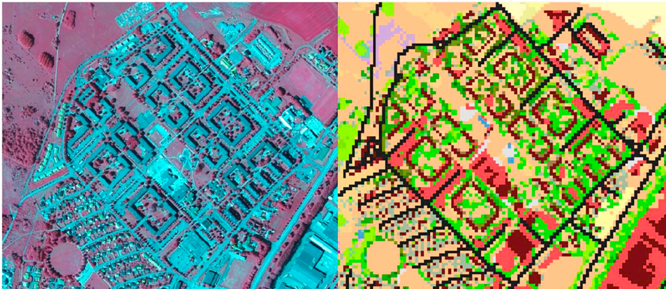
Figure 7.7 Example of urban green areas from the Swedish National Land Cover Mapping (NMD), where the land cover is integrated with moisture regime, showing the grassy areas in three different hues of beige/orange, depending on the degree of moisture, and trees and shrubs are differentiated into coniferous, deciduous, or hardwood deciduous and are shown in green hues.
