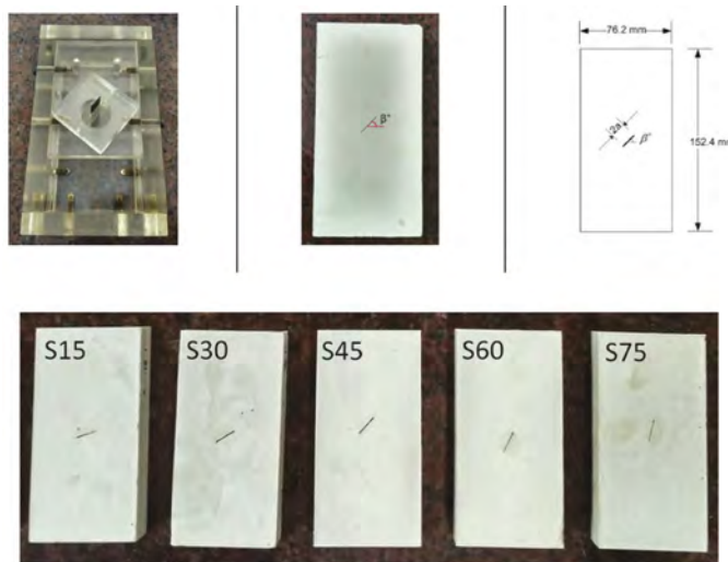
Figure 1. a) Specimen preparation mould with prepared gypsum specimen with single flaw of different angles.
