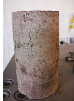
Figure 6. Failure of soil-kaolinite geopolymer UCS test specimen.
