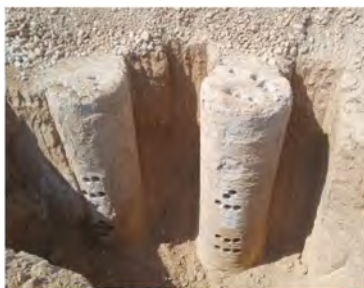
Figure 1. General view of soil-cement column samples for core sampling .
