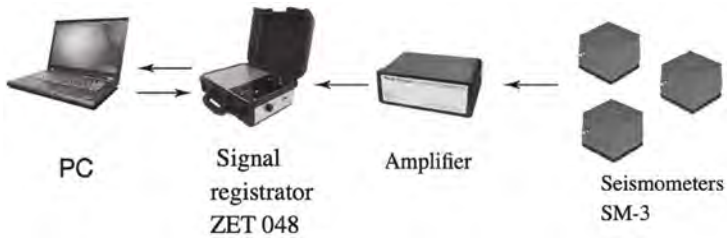
Figure 1. Test devices set.
