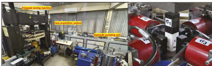
Figure 3. (a) Polyaxial testing machine installed at IIT Delhi, and (b) True triaxial loading setup of rock specimen.
