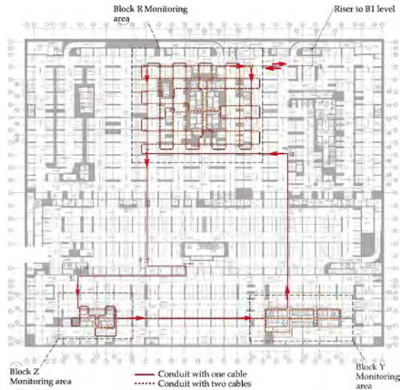
Figure 3. Part plan of cable routing in block R monitoring area on B4 raft.
