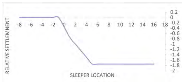
Figure 2. Relative settlement at sleeper location.
