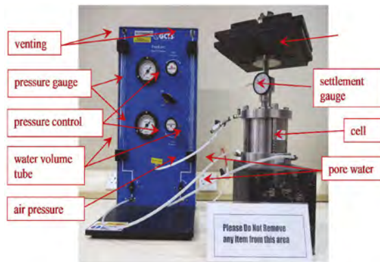
Figure 6. Fredlund cell set up during WRC testing.
