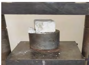
Figure 3. Destruction of the sample when determining the ultimate compressive strength.
