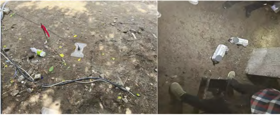
Figure 9. Measuring ground vibrations by placing Accelerometers and Geophones.
