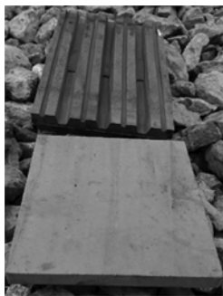
Figure 1. Standard CP-204-M-APC gasket (standard, top) and Sylodyn NF high-elasticity gasket (experimental, bottom).
