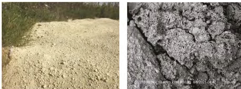
Figure 1. Light technogenic soil: left – general view; right - micrograph of a chipped silicate pellet obtained by utilizing a sulfur-alkali solution through interaction with trepel.
