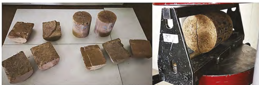
Figure 8. Failure of ITS test specimens of soil-kaolinite-based geopolymer mixture.
