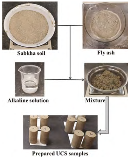
Figure 2. Procedure for preparation of geopolymer-treated samples.
