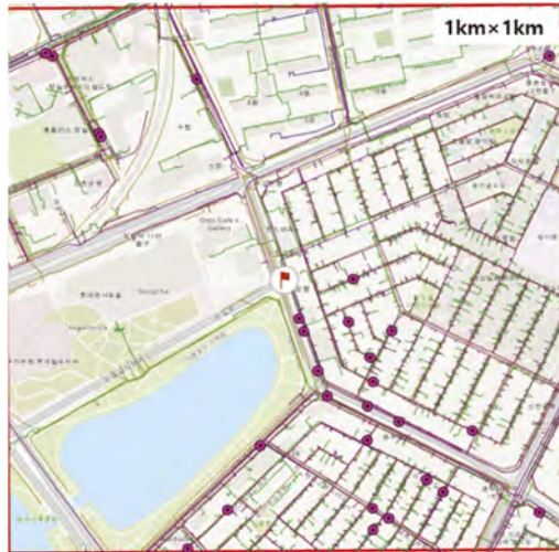
Figure 2. The 1\text{km} \times 1\text{km} Map of analysis area and 29 ground subsidence locations with magenta circle symbol (Choi et al. 2021).
