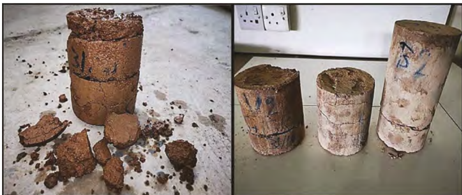
Figure 10. Soil stabilized using kaolinite geopolymer after two cycles of W-D conditions test.
