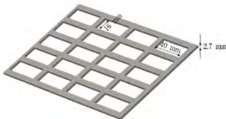
Figure 1. Geogrid detail dimension.
