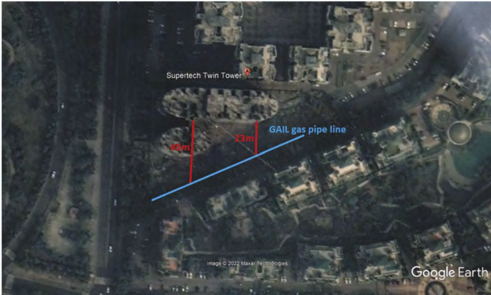
Figure 3. Layout of GAIL gas pipeline within the compound of SuperTech Twin Tower.
