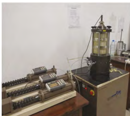
Figure 1. DYN77S dynamic triaxial test apparatus. Figure 2. Curve of cyclic loading.
