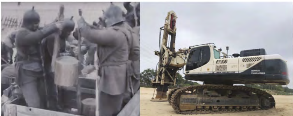
Figure 1. Compacting in the past, stomping (left), and now, impulse compactor (right).
