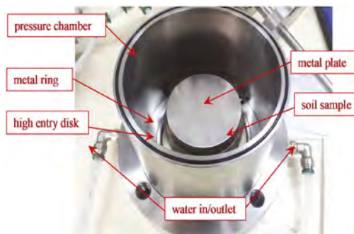
Figure 7. Open Fredlund cell before WRC testing is started.
