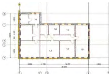
Figure 9. Merchant Senokosov's House. Plan of the 2nd floor, measurement of the building, 2016.
