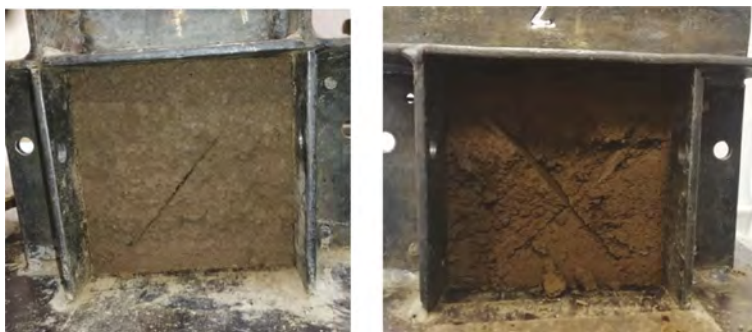
Figure 2. Samples with cracks in the equilibrium planes: a) with one crack; b) with two intersecting cracks in two equilibrium planes.
