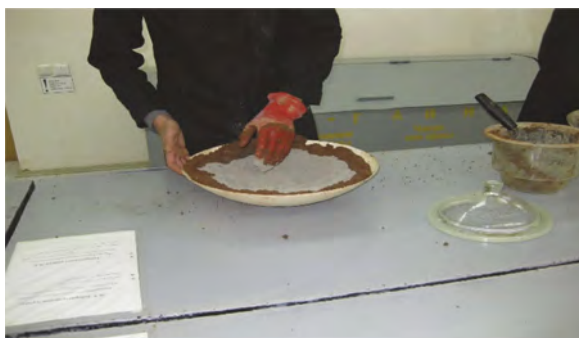
Figure 4. The process of adding quicklime to the soil surface.
