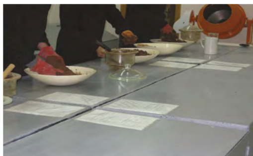
Figure 3. The process of preparing soil with different moisture content in laboratory conditions.
