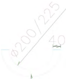
Figure 13. Semi-circular chute drain.
