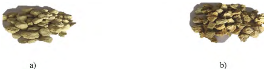
Figure 6. Crushed stone modified with resin (a); crushed sulfur stone modified with styrene (b).
