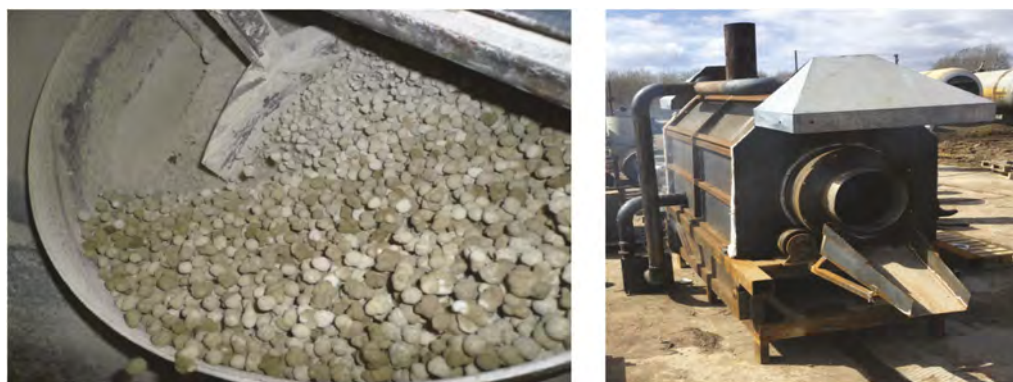
Figure 2. Production of a technogenic soil: left - production of raw pellets from sulfur-alkali waste and trepel in a pan pelletizer, right – the drum kiln.
