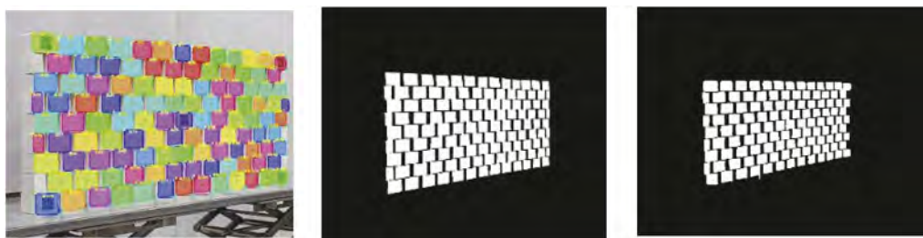
Figure 3. An example of the blocks trained and detected for the laboratory experiment: (a) detected image, (b) trained mask, (c) detected mask.
