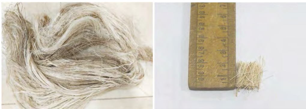
Figure 5. a. Banana fibre collected from local sources. b. Banana fibre after cut into 2 cm.
