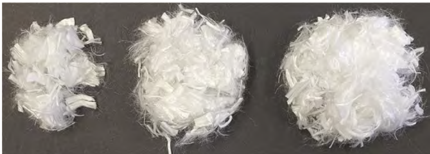
Figure 4. The polypropylene fibers with 12 mm longest added to the soil in a mass ratio of 0.1%, 0.2% and 0.3% to the dry mass of the compacted soil.
