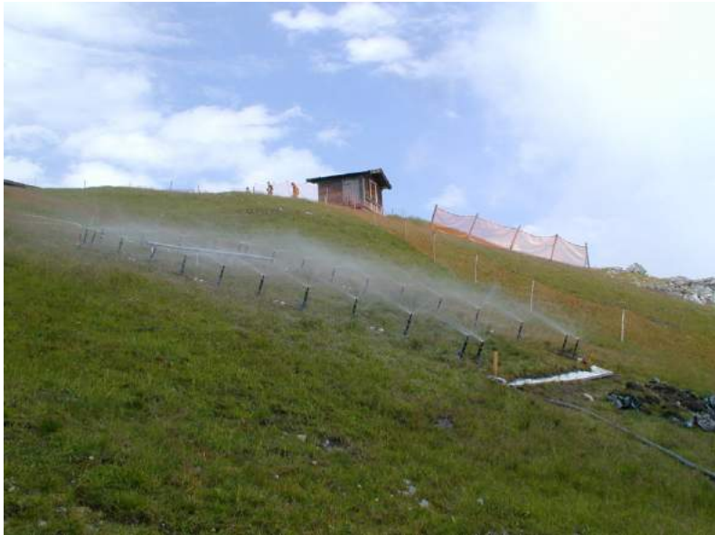
Figure 8: Sprinkling irrigation experiment at one of the test plots of 100 m 2 each, St. Anton 2005.
