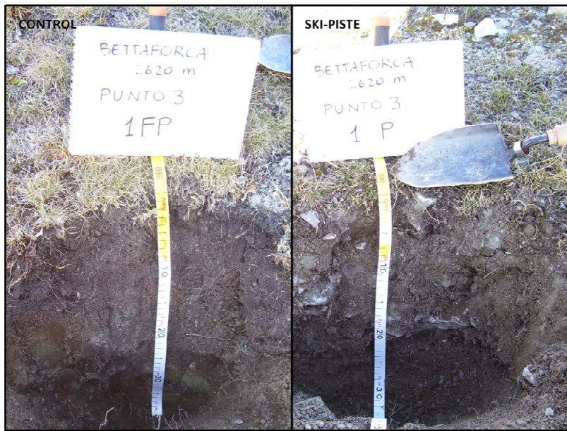
Figure 3: Effect of ski-run construction on the abundance of rock fragments in the Italian Western Alps (Monterosa Ski Resort, NW-Italy, 2620 m a.s.l.).
