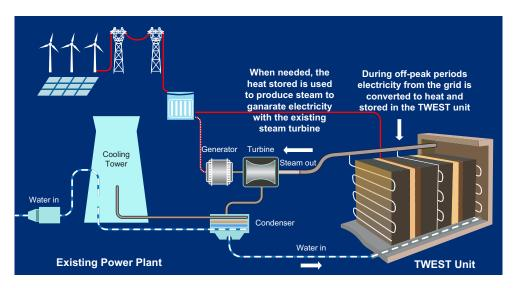
*Figure 15.2* Repurposing thermal power plant illustration. *Source:* E2S Power.
