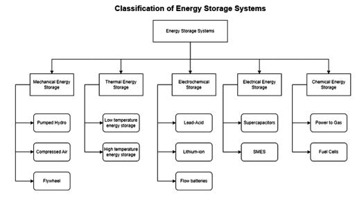
*Figure 15.1* Classification of energy storage systems based on the form of energy stored. *Source:* Compiled from https://www.sciencedirect.com/science/article/abs/pii/S0306261916308728 and https://ieeexplore.ieee.org/document/8580457.
