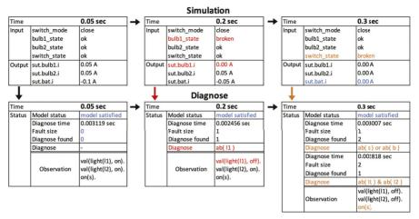
Simulation and diagnose output results based on the electrical two-lamps circuit with a broken bulb after 0.2 seconds and a broken switch at 0.3 seconds. The upper tables illustrate the simulation input/output signals, which are used as observation for the diagnose (lower tables) part. Based on the given observations for the three selected time steps, different diagnose results are obtained.
