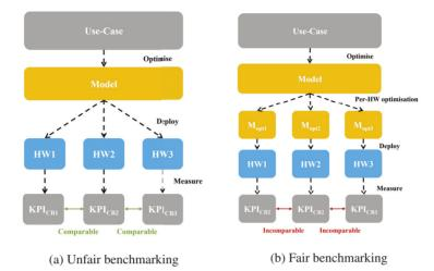
**Figure 1.1** Benchmarking fairness. (a) Unfair benchmarking: the KPIs are comparable, but the benchmarked hardware platforms are not exploited to their full potential. (b) Fair benchmarking: the hardware platforms are exploited to their full potential, but the resulting combined KPIs ( $KPI_{CB}$ ) are not comparable.
