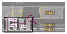
Figure 4.13 Example cross-section image with annotated metal and contact/VIA features
