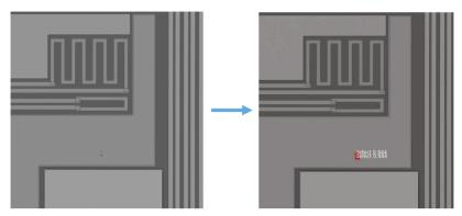
Figure 5.4 Example of binary classification of wafer defects: defect vs background
