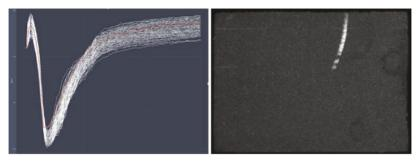
**Figure 6.1** *Left:* Curve with abnormal minimum position (red) in comparison to normal ones (white) of recorded sensor data during wirebonding process. *Right*: shows an example of abnormal OOI image with shown crack on the surface.
