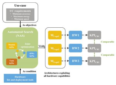
**Figure 1.3** Benchmarking pipeline based on use-cases. An automated search finds the best possible model exploiting the performance offered by each target hardware platforms. The resulting combined KPIs are comparable.
