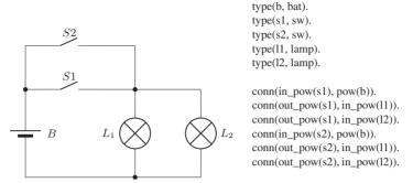
**Figure 14.4** Another simple electric circuit comprising bulbs, switches and a battery. This circuit is an extended version of the circuit from Figure 14.1. On the right, we have the structural model of this circuit in Prolog notation.
