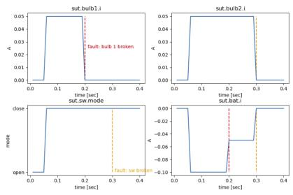
**Figure 9.3** Simulation showing the measured signal output of the two bulbs, switch and the battery. For this example a fault injection (broken) in bulb 1 after 0.2 seconds (red indicator) and a fault injection (broken) to the switch after 0.3 seconds (orange indicator) is initiated.
