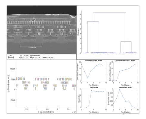
**Figure 4.14** Example cross-section image (upper left). The polygonised VIA objects are shown (lower left). A dendrogram is shown for the relative distances of the y-coordinates of the single objects (upper right). Finally, the results of the utilised cluster evaluation techniques are presented (lower right).
