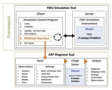
**Figure 9.2** Illustration of the simulation and diagnose environment as well as the overall operating principles. The framework of the FMU Simulation Tool provides an interface to enable the integration of a diagnose tool and/or other methods. The models can be substituted by any others in the provided framework.
