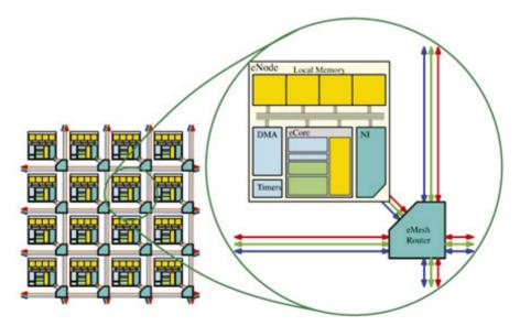
**Figure 2.1** Overall scalable architecture of Epiphany-III [1].
