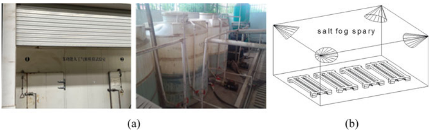
Fig. 2.2 Artificial climate test box: a photo, b schematic
