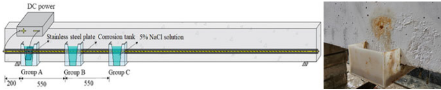
Fig. 6.15 Local corrosion location of specimens (Unit: mm)
