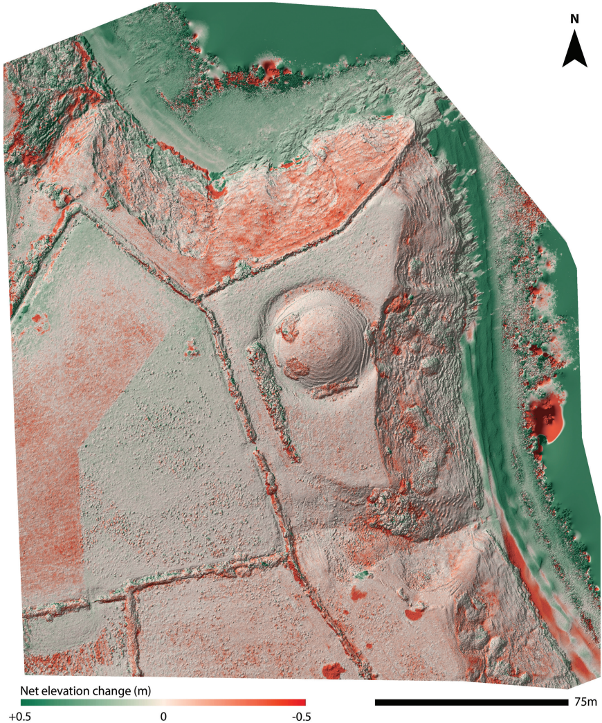
FIGURE 9.15 ‘DEM of Difference’ (DoD) analysis for UAV-derived DEM between 2018 and 2019 at Glascarrig Motte and Bailey site on the County Wexford coastline.
