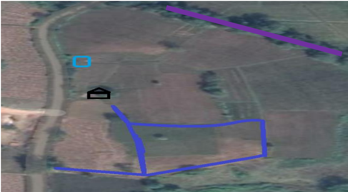
Figure 15. Bhoomi site before planation, with well (light blue), trenches (dark blue) and canal (purple).
