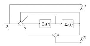
Fig. 5.12. Encoder of the recursive convolutional code to be compared with the non-recursive case of Fig. 5.11.
