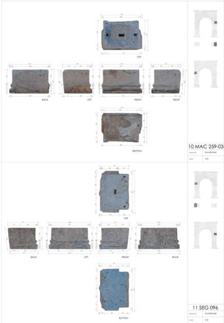
Fig. 14. A stone catalogue is prepared comprising of orthographic documentation of each architectural piece, derived from the 3D models.
