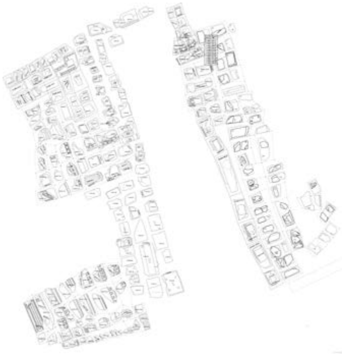
Fig. 13. Platform plan at the end of the organisation of blocks. Attention should be paid to providing space to study the blocks and allowing access to each piece with the crane.
