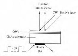
Fig. 7.4 Experimental arrangement used for phonon wind experiments.
