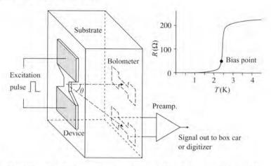
Fig. 2.3 Geometry of a phonon emission experiment. Two bolometers (phonon detectors) are shown, one is directly opposite the active area of the device and one is at angle  $\theta$  to the device normal. The inset shows the resistance R of a typical aluminium bolometer around its superconducting transition and the steady-state bias point is indicated.
