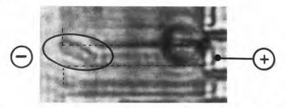
Fig. 3.11 He film image of a 2DEG showing QHE breakdown within a 200 µm wide strip connecting two large areas. The ellipse shows the helium drop that has formed above the region where breakdown has occurred [54].
