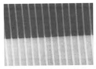
Scanning electron microscope (SEM) micrograph of part of an array of freely suspended Si<sub>3</sub>N<sub>4</sub> wires projecting over the Si support and the anisotropically etched hole. The wires are about 1 μm apart. (After Lee et al. [5].)
