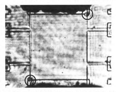
Fig. 3.10 He film image of a 2DEG Hall bar. The helium drops at the two diagonally opposite corners show the location of the hot spots and their diameters provide upper limits to the hot spot sizes [47].
