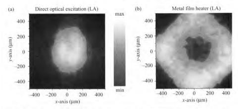
Fig. 2.19 (a) Image of the LA phonon emission by optically excited carriers in a (001) GaAs quantum well. The bolometer is located at the centre of the image. (b) For comparison, the image for laser heating of a metal film on a GaAs substrate. It is clear that the emission by 2D electrons is channelled into a narrower range of angles close to [001] due to in-plane (2k<sub>F</sub>) momentum conservation.
