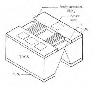
Fig. 8.5 Schematic layout of device with freely suspended Si<sub>3</sub>N<sub>4</sub> wires for one-dimensional phonon transport studies. (After Lee *et al.* [5].)
