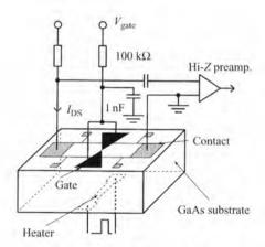
Fig. 4.11 The experimental arrangement for measuring the absorption of non-equilibrium phonons by a QWR.
