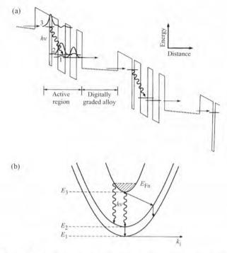
**Fig. 6.20** (a) Energy levels of a section of a quantum cascade laser: electrons are injected into level 3, make a radiative transition to level 2 followed by a LO phonon-assisted transition to level 1; (b)  $E(k_{\parallel})$ : radiative and phonon-assisted transitions are shown by wavy and straight arrows respectively [132].
