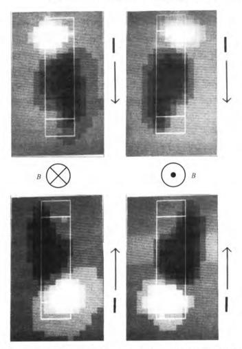
Fig. 3.13 Phonoconductivity images of the two-terminal resistance of a Hall bar in the IQH state for the four possible permutations of magnetic field and current directions. The dark (light) areas correspond to an increase (decrease) in resistance [67].
