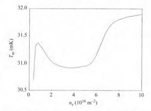
Fig. 2.29 Temperature rise measured on a resistance thermometer located directly opposite an Si-MOS device as a function of  $n_s$ . The 2DEG is heated by a constant electrical power input of 47  $\mu$ W.
