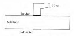
Fig. 4.16 The experimental arrangement for measuring the phonon emission from an array of QWRs.
