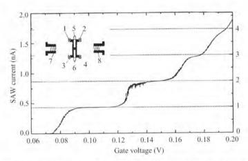
**Fig. 6.31** The current passing through a pinched-off ID channel produced by an SAW as a function of gate voltage (after Janssen and Hartland [186]). Inset: a typical experimental arrangement showing the ohmic contacts to the ID channel, 1–4, split gate, 5–6, and SAW transducers, 7–8 [182].
