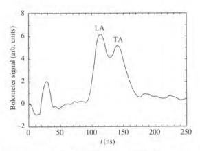
**Fig. 2.4** Typical bolometer signal for phonon emission by a 2DEG in a GaAs quantum well. The signal in the first 40 ns after the start of the excitation pulse at time t=0 is due to electromagnetic breakthrough of the pulse. The longitudinal (LA) phonons arrive at 90 ns followed by the transverse (TA) phonon pulse at 130 ns.
