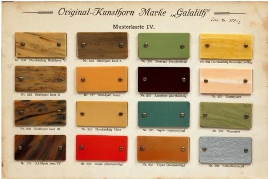
FIGURE 19.1 'Original-Kunsthorn Marke "Galalith"'. Sample card no. IV, showing the different colour variants of Galalith or 'milk stone', a new material synthesised of milk proteins and produced in the early twentieth century to imitate horn and ivory. Mustertafel mit Galalith-Erzeugnissen Nr. 4, Internationale Galalith-Gesellschaft Hoff & Co. Harburg (Hamburg) 1928–1930 © TECHNISCHES MUSEUM WIEN
