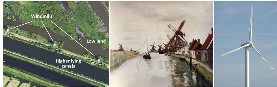
Figure 3.2: Left: Windmills along a canal in Kinderdijk, Holland (satellite photo: Google Maps), pumping water from low lying land into higher up canals. Center: Windmills along a canal (painting by Claude Monet, 1871). Right: Modern wind turbine.
