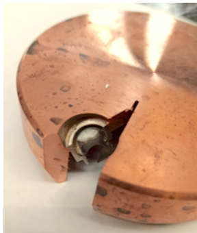
Fig. 5.2: Photo of a test weld of a test piece cutted on the cable feed-through.
