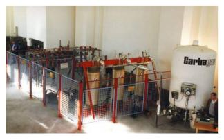
Figure 9.1.1: 10 kV, 70 A shielded core type superconducting fault current limiter from ABB [Paul1997]
