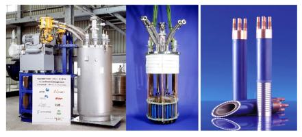
Figure 9.1.2: 10 kV, 600 A CURL10 fault current limiter (left) and Bi2212 bulk material current limiting element (right) [Bock2005, Kreutz2005]
