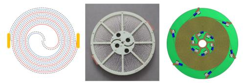
Figure 4.3.1: Schematic diagram of a bifilar coil (left) and a designed current limiter module with hightemperature superconductors [Kraemer2021] (middle). On the right a multifilar arrangement with three bifilar coils in parallel [Noe2012]
