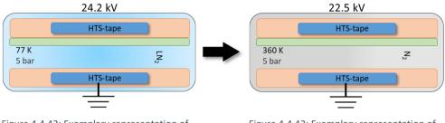
Figure 4.4.42: Exemplary representation of the plane layered arrangement under LIC stress during normal operation
