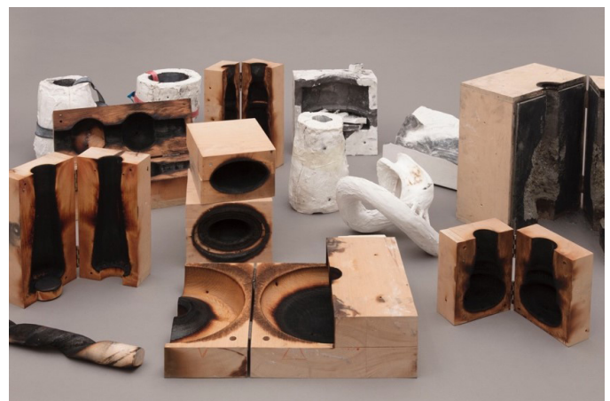
Figure 5. The variety of different moulds produced at the wood workshop of Lucerne School of Art and Design: most of them on the CNC milling machine in massive beech, others in plaster or even sand Image: Andri Stadler
