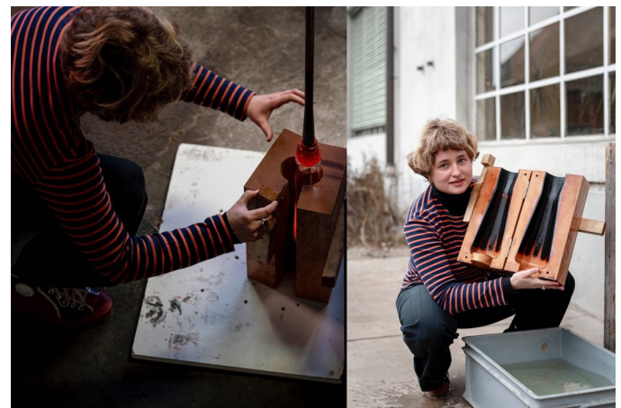
Figure 3. Glass blowing at the Open Glass Studio with help of a digitally milled mould Images: Raisa Durandi
