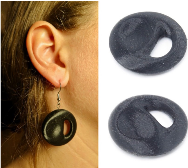
Figure 2. FDM earring printed in different orientations. Design, 3D print, and photos: Ricardo Simian, 2022
