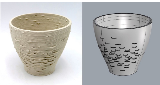
Figure 3. 3D printed clay cup with semi-regular patterns alongside the 3D model which was fed into the printed. Design, 3D print, and photos: Ricardo Simian, 2022
