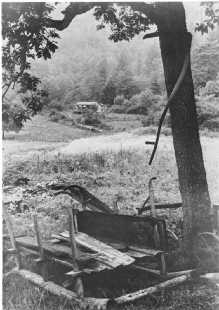
A timber sled used in skidding logs and for other hauling purposes on steep hillsides
