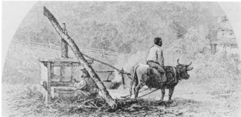
A sorghum mill extracts the juice, which is then boiled down in the iron pot
