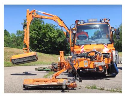
Figure 1.1: An exemplary image of a large vehicle manipulator with three working attachments.
