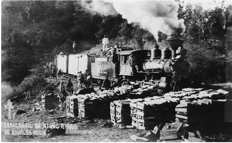
Figure 1.1. Ajuno-Ario de Rosales Railway, ca. 1910. The firewood stacked in the foreground is fuel, as the tender filled with firewood suggests. Universidad Michoacana San Nicolás de Hidalgo, Instituto de Investigaciones Históricas, Sánchez Díaz Collection.
