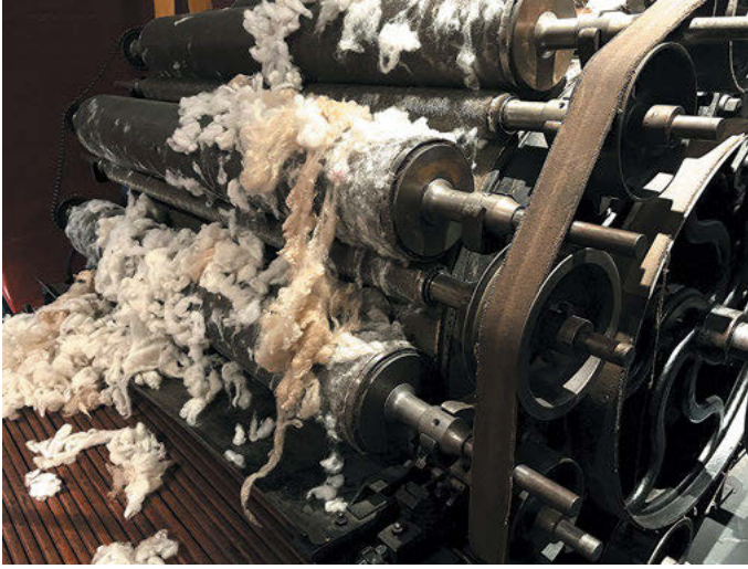
Figure 1.3: Carding machine to clean and disentangle wool to produce a continuous web for subsequent processing (photo Léo-Paul Dana).
