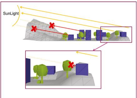
FIGURE 7.9 Measuring view composition (top) and analysing sunlight and shadow computations (bottom) at different scales
