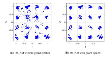
Figure 6.13: 16QAM symbols without/with guard symbols
