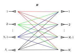
Figure 2.4: Channel model for a multi-antenna system.
