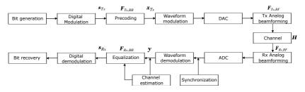
Figure 3.1: The general signal processing chain in this dissertation.
