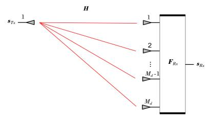
Figure 2.10: Structure of SIMO system with spatial diversity at Rx.
