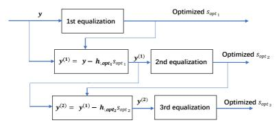
Figure 3.4: Computing procedure of SIC-based equalization.
