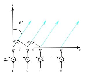
Figure 2.6: Phased array beamforming principle.
