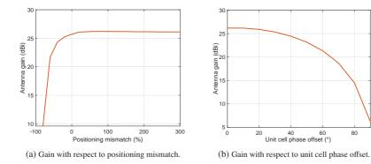
Figure 4.12: IRS beamforming simulation with distortions.
