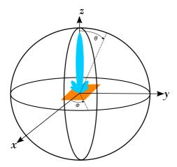
Figure 2.1: 3D coordinate system for antenna analysis.
