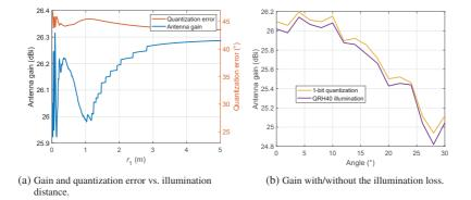
Figure 4.10: IRS beamforming simulation considering illumination properties.
