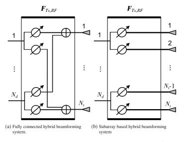
Figure 2.15: Hybrid beamforming system architectures based on [MRH<sup>+</sup>17].
