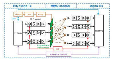
Figure 7.2: System model for PM hybrid MIMO beamforming.
