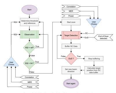
Figure 6.17: Working principle of the control angle block.
