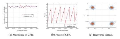
Figure 8.3: Channel estimation results and signal recovery results for IRS assisted MIMO.
