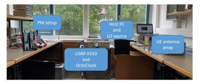
Figure 7.3: Measurement environment for the IRS hybrid MIMO beamforming system for singleuser scenario.
