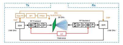
Figure 6.1: The block diagramm of SISO communication system using IRS beamforming from [LWE+20].
