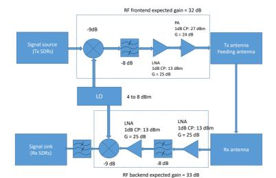
Figure 5.6: Structure of RF frontend and backend module.
