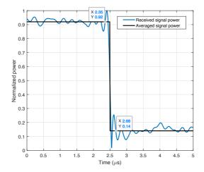
Figure 6.11: Settling time of the IRS beam switching.
