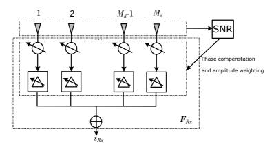
Figure 2.11: Structure for maximal ratio combining (MRC).
