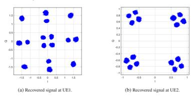
Figure 7.18: Multiuser recovered symbols with interference.
