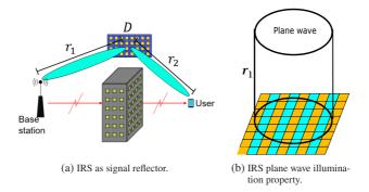
Figure 4.7: Farfield IRS illumination principles.
