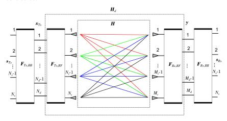
Figure 2.14: System model with hybrid beamforming.
