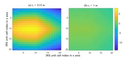
Figure 4.11: Power distribution imbalance at different  $r_1$ .
