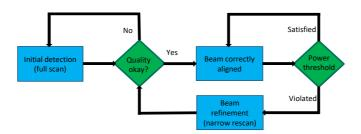
Figure 6.16: The flow graph of beam management.
