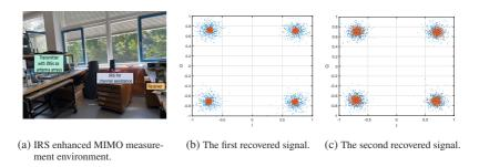
Figure 8.6: Recovered signals for RIS enhanced MIMO system.
