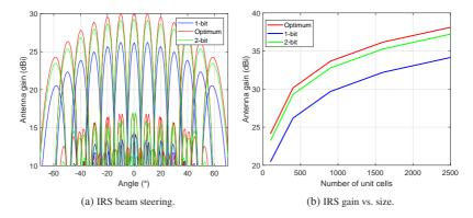
Figure 4.9: IRS beamforming simulation using different phase resolutions.
