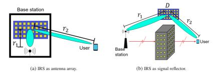
Figure 1.1: IRS application types.
