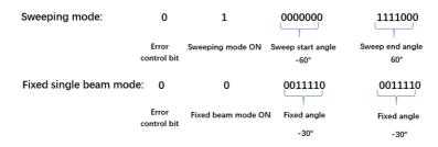
Figure 4.5: Command structure for IRS coding pattern.
