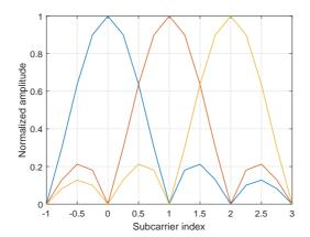
Figure 3.6: OFDM Modulated signals in frequency domain.
