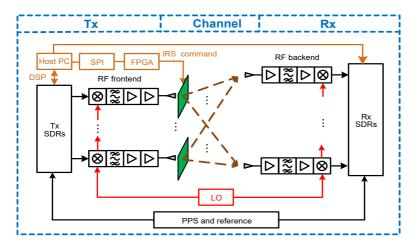
Figure 5.1: The general model for IRS-based communication systems.
