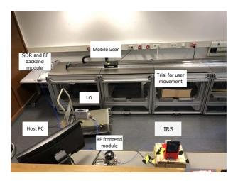
Figure 6.15: Indoor system setup of IRS mobile communication tracking.
