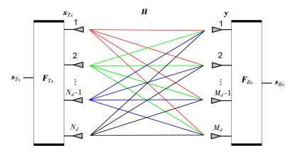
Figure 2.13: Structure of MIMO system with spatial multiplexing.
