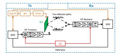
Figure 6.6: The block diagram of IRS wireless communication system under multipath SISO scenario
