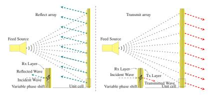
Figure 2.7: Reflect array and transmit array.
