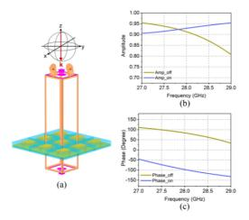
Figure 4.3: IRS unit cell simulation environment and results from [WXZ<sup>+</sup>21].
