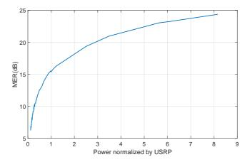
Figure 7.11: An example for relationship of SDR normalized power and System MER.
