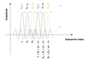
Figure 7.1: Theoretical interleaved OFDM subcarriers at Rx.
