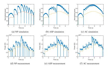
Figure 6.22: Figures for IRS tracking system performance analysis. (a) to (c): Simulation results. (d) to (f) measurement results. Blue curves denote the Rx power and yellow curve denotes the tracking observation.
