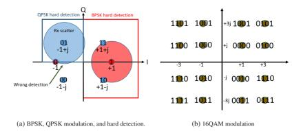
Figure 3.2: Digital modulation schemes in the constellation diagram.
