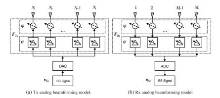
Figure 2.5: General model of analog beamforming.
