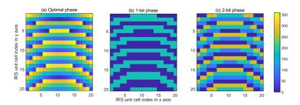
Figure 4.8: IRS phase distribution with different resolutions.
