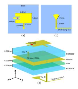
Figure 4.2: IRS unit cell design in this dissertation from [WXZ<sup>+</sup>21].
