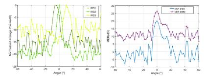
(a) Anaglog beam training results for 3 IRSs at the Tx. (b) Comparison of SISO and MISO beam training.
