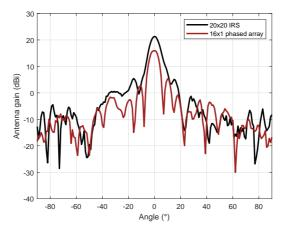
Figure 4.14: Comparison between phased array and IRS
