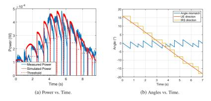
Figure 6.20: Tracking observation for v = 10 m/min,  $\sigma_t = 0.6$ , and  $k' = 16^{\circ}$ .
