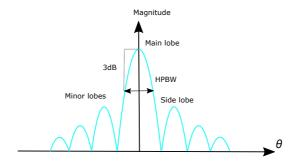
Figure 2.2: 2D plot of the antenna pattern lobes.
