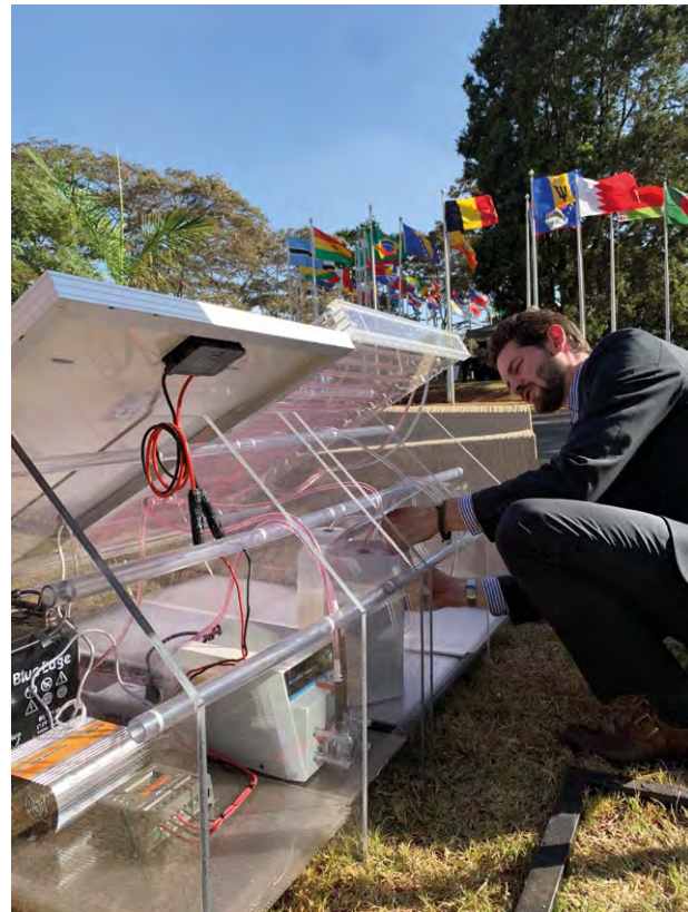
4 & 5. SEWR Embodiment: Incorporating plant-based edible photosensitisers into household water treatment practices that provide a visual indication of safe drinking water when the fluid runs pink to clear. Demonstration at UNEP Headquarters, Nairobi, Kenya, 2019. © Yale Center for Ecosystems + Architecture.
