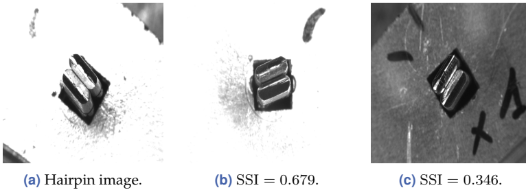
Figure 3.27 Comparison of the SSI. The subfigures (b) and (c) are compared with the image in (a)
