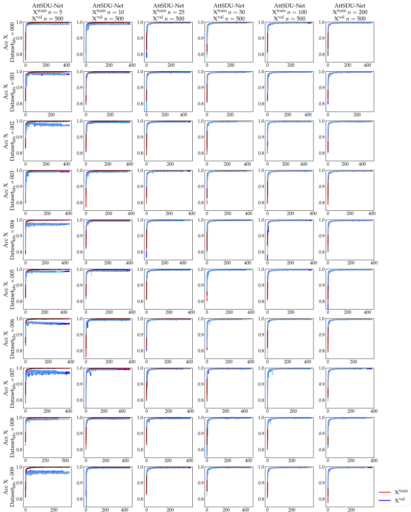
Figure A.6 Accuracy of the AttSDU-Net. In red are the results on the data set \mathbb{X}^{\text{train}} and in blue for \mathbb{X}^{\text{val}} . The x-axis represents the progression of epochs during the training process. Five model were trained on each data split from scratch.
