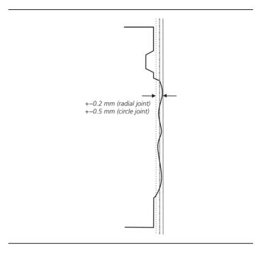
Figure 204.4 Combined tolerances for radial joint (204.4.1 (j) and (k))
