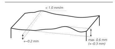
Figure 204.5 Establishment of the theoretical joint plane from the survey grid (204.4.3.5) and rate of inclination derivation
