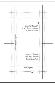
Figure 204.3 Acceptable tolerances for joint surface offset from theoretical plane in radial plane (204.4.1 (j) and (k))
